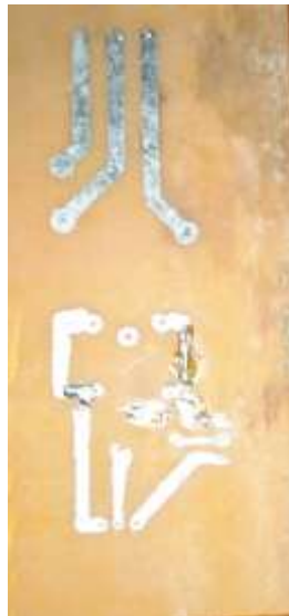
Figure 2: Track Defective PCB
